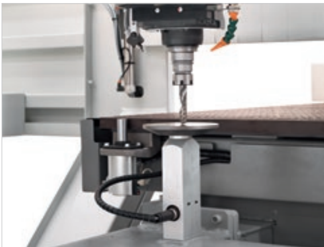
The contact pre-setter automatically measures the length of tools up to 130 mm in diameter. This greatly reduces the machine tooling time and eliminates any risk of mistakes by the operator.
