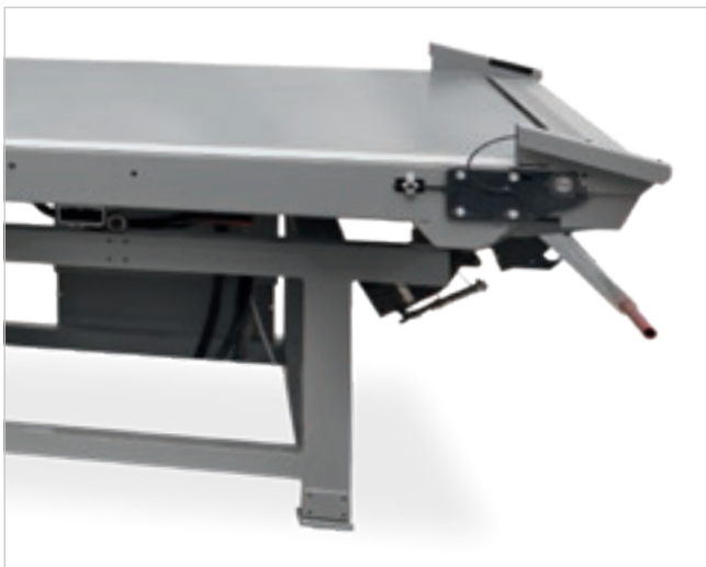
Intake manifold positioned at the end of the belt.
