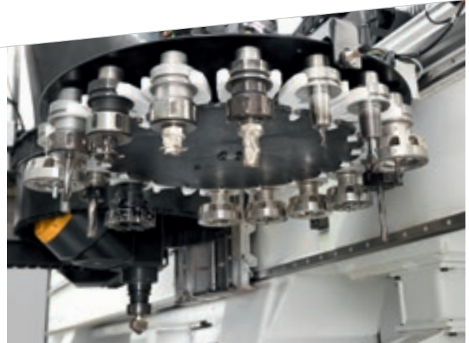
New tool magazine with 18 places: spacious and fast, for those wanting to try out different products with the 5-axis unit.
