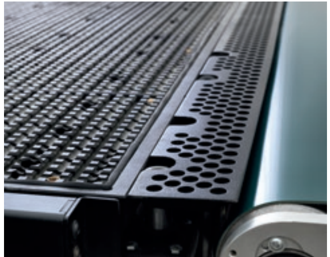
Chip removal system positioned between the machine and the unloading belt, guaranteeing optimal sheet cleanliness.
